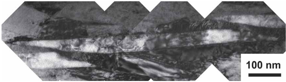
Fig.5 TEM bright-field image of bainite sub-unit structure obtained from isothermal transformation at 300°C for 4 hours.
