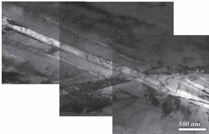
Fig.7 TEM bright-field image of bainite structure obtained at 300°C for the first 2 hours and than heat treatment at 200 °C for 2.5 days.
